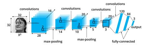
Fig. 2. Proposed structure of deep neural network (referred as N2 in Table 1) for head orientation estimation. It uses  $32 \times 32$  pixels gray scale image as an input. The output is head orientation  $(\psi, \theta, \phi)$ .
